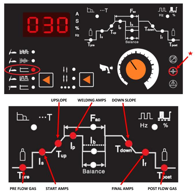
Set parameters as follows using control panel image above as reference:
