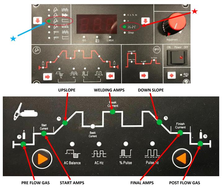
Set parameters as follows using control panel image above as reference:
